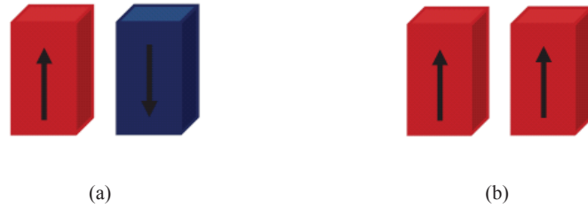
Figure 2.9 (a) Definition of logic '1' and '0' for nanomagnets and (b) Metastable states for coupled pairs.
